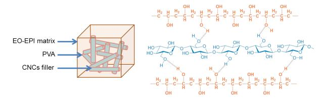
Schematic representation of the proposed system for PVA-enhanced mechanical properties of EO-EPI/CNC nanocomposite.
